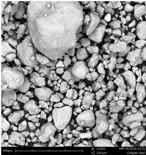
Fig. 1: SEM Micrograph of a Conventional Abrasive (Silica) Particle Size Distribution = 1 to 100µm.
